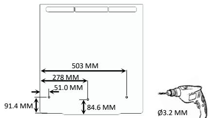
2. Fix the front stopper plate with help load spreading rivet/flower type rivet.
