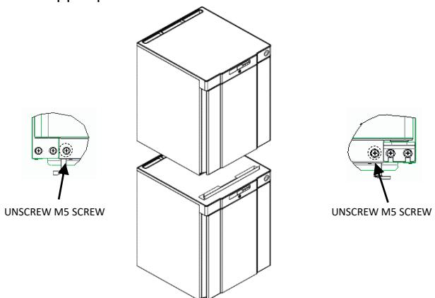
4. Fix top unit with front stopper plat using M5X15 existing screw of top unit.
