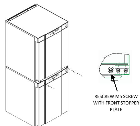
5. For back stopper plate, drill 3.2mm diameter holes (position back stopper plate and transfer its holes to cabinet. Fixed back stopper plate with help of T5X15 Screws, 4 number each.
