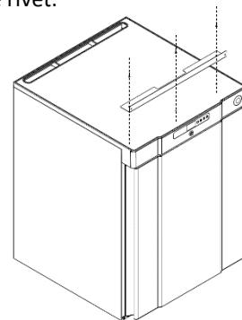
3. Unscrew and remove M5X15 screw from top unit, Place top unit on table top and align the holes to match with the front stopper plate hole.
