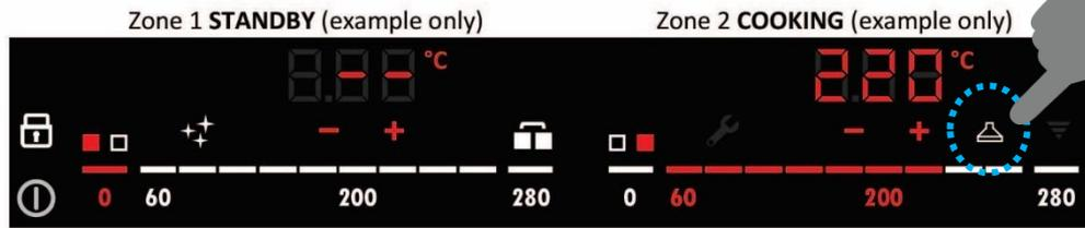
Manual Fan Speed function still not active, meaning that the user never touched the H2H key since the UI is in ON state.
