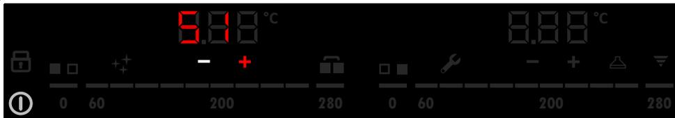
From here user can press "-" key to switch to "S2" service utility page, press On/Off key to exit SERVICE MENU or wait 8 sec to automatically exit from SERVICE MENU .
