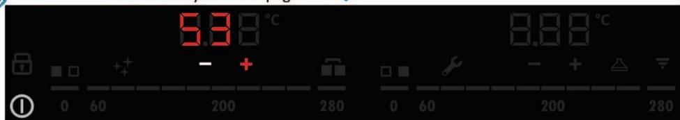
From here user can press "-" key to switch to "S4" service utility page, press On/Off key to exit SERVICE MENU or wait 8 sec to automatically exit from SERVICE MENU.
