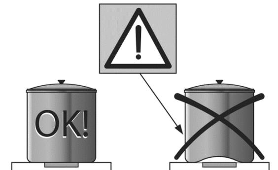
Do not use empty pots or pans on the appliance as they can quickly (in a few seconds) reach very high temperatures.
