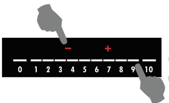
**POWER MANAGMENT** the power output regulation can be set by pressing the sliding bar or pressing on the “plus / minus”
