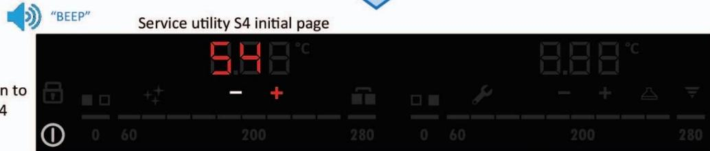
From here user can press "-" key to switch to "Demo mode" page, press On/Off key to exit SERVICE MENU or wait 8 sec to automatically exit from SERVICE MENU.
