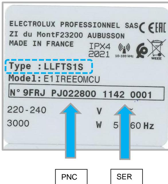
SERIAL NUMBER (PRODUCTION DATE) is necessary to find the correct spare part or to ask tech. support.
