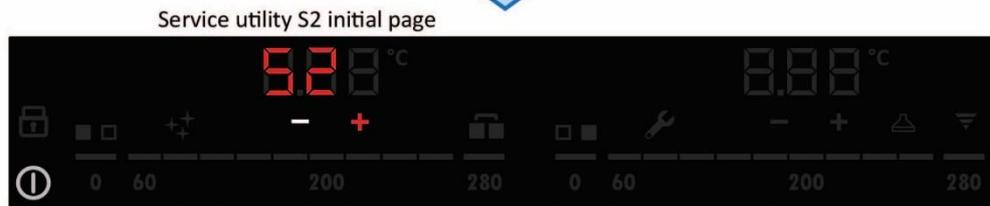
In this case the UI automatically returns to the Service utility S2 initial page without showing the test result.
