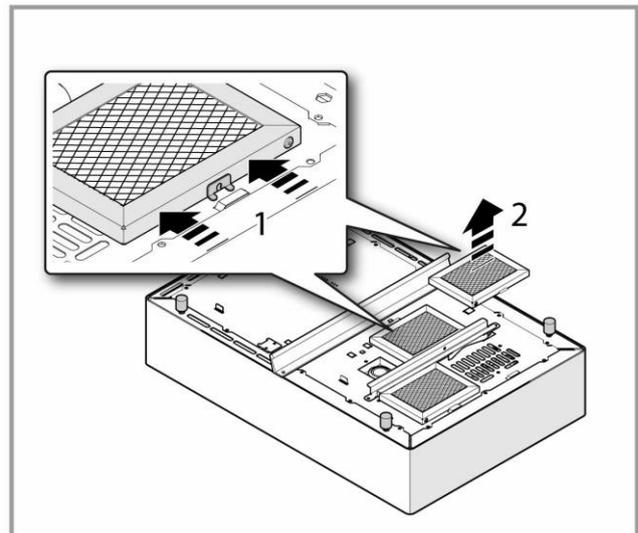
**The air filters:** can be washed separately or inserted into a dish washing machine, dry carefully or leave to dry on a dish rack or towel.
