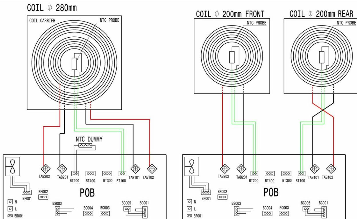
The appliances are not driven by a thermostatic function, they work by emitting power depending on the setting level on the u.i. . The temp.sensor is therefore sensing the coil temperature to protect the component in case of overheating.
