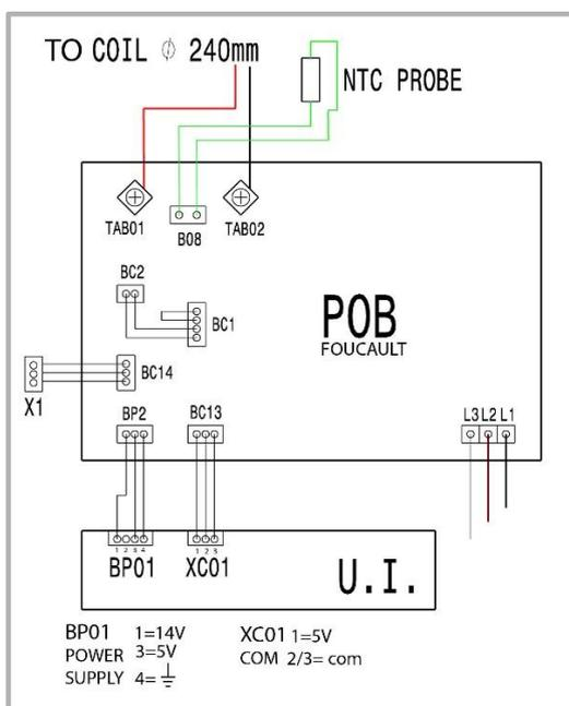
To check if the inner voltage adaptor is functioning . The voltage adaptor is a component located inside the generator and cannot be replaced, but It can be checked. Locate the connectors , check the indicated pins; If there is no voltage (12v) on these pins the inner voltage adaptor is broke.
