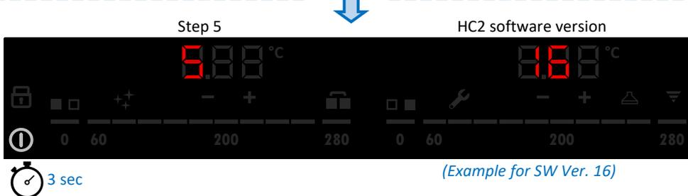
This step is present only for configurations with two power boards, meaning for Double Zone Frytop.
