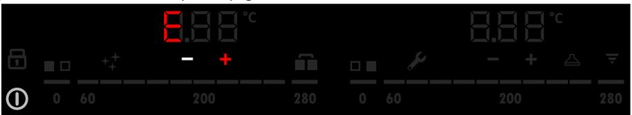
User can press "-" key to switch to "Beep mode" setting page, press "+" key to restart alarm history visualization, press On/Off key to exit CUSTOMER MENU or wait 8 sec to automatically exit from CUSTOMER MENU .
