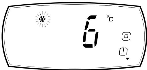
To activate and deactivate the appliance touch Program button for 3 seconds to unlock the display
