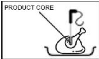
When the product thickness allows, use always the temperature needle probe in order to know the exact temperature reached at the product core. It is suggested to not interrupt the blast chilling cycle before it has reached the temperature of **+3 °c**, in positive cycle and **-18°C** for the negative cycle.
