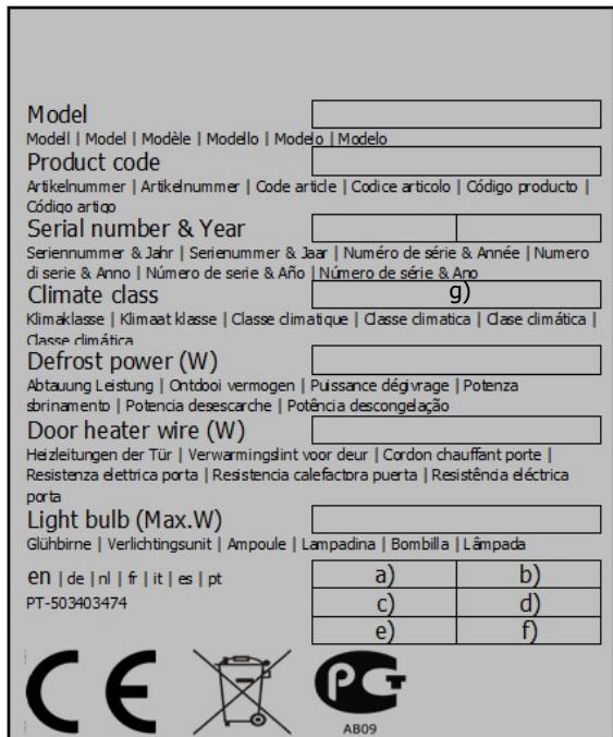
The rating plate on our mini cold rooms is located inside the door. It includes the main technical data about the equipment and it identifies the MODEL and SERIAL NO., which are vital pieces of information for any queries to the manufacturer.
