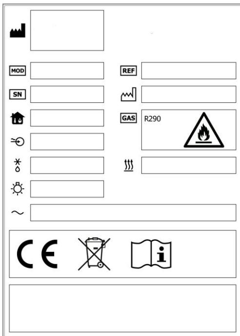
The rating plate on our equipment is located inside the equipment, on the left side panel. It includes the main technical data about the equipment and it identifies the MODEL and SERIAL NUMBER, which are vital pieces of information for any queries to the manufacturer.
