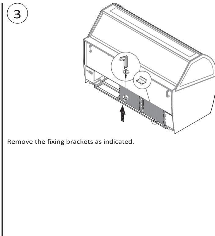
Remove the fixing brackets as indicated.
