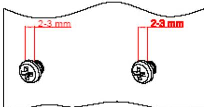
Make sure the distance between the screw head and the wall is 2-3 mm.
