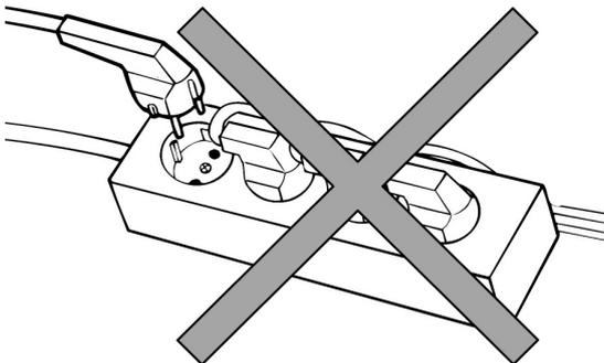
The appliance should not be connected to a multipoled distribution socket.
