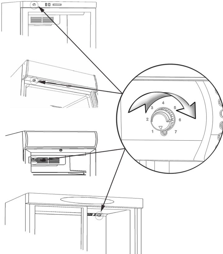
Depending on model the thermostat can be placed as follows:
