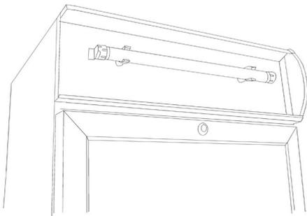
Push carefully the canopy plate in place and remount the end piece of the canopy.
