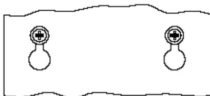
Make sure the screws fit perfectly into the wall fitting.
