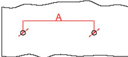
Drill 2 holes with a diameter of 8 mm and a depth of 40 mm and a distance as shown on the drawing (A).
