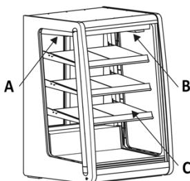
A - Air suction. Never block the suction. Air is sucked in and cold air is circuated inside the refrigerator.
