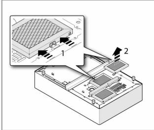
**The air filters:** can be washed separately or inserted into a dish washing machine, dry carefully or leave to dry on a dish rack or towel.
