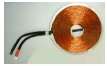
At the center of each coil is located the temperature probe that acts also as safety probe.
