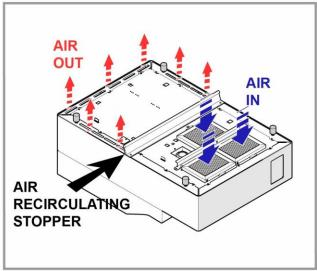
The appliance is a high performer and will require a big amount of fresh air to cool its internal components.
