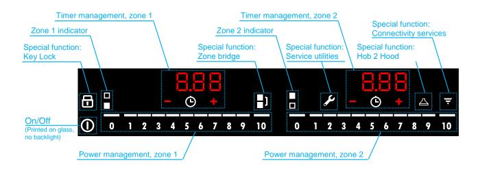
ON /OFF Touch the button: the griddle will turn on; a lamp test will occur, and the zone will then be ready for temp regulation/setting.
