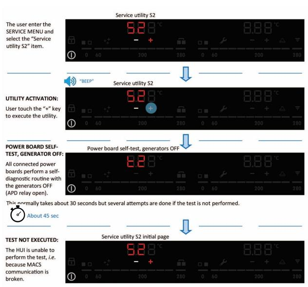
In this case the UI automatically return to the Service utility S2 initial page without showing the test result.
