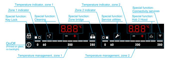
ON /OFF Touch the button: the griddle will turn on; a lamp test will occur, and the zone will then be ready for temp regulation/setting.
