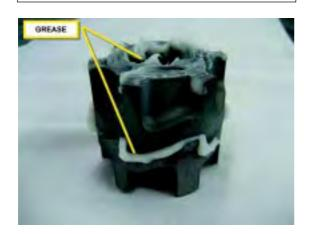
NOTE. Install the upper bearing into the ice breaker starting by the radial portion that must be fitted with the flat surface facing up. Apply some lubricant (grease) on the upper surface then install the rollers cage with the smaller openings of the same facing up so to leave a small gap between plastic cage and flat surface of the botton portion of the bearing (see drawing).
