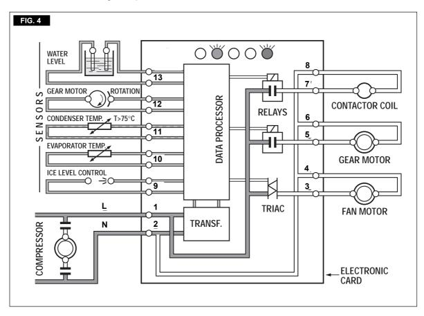
This will cause a gradual decrease of the water level in the float reservoir and as soon as the level gets below the two vertical metal pins, the flaker stops to operate (compressor first and 3' later the gear reducer) and the ELLOW warning LED will glow to signal the shortage of water (Fig. 4)
