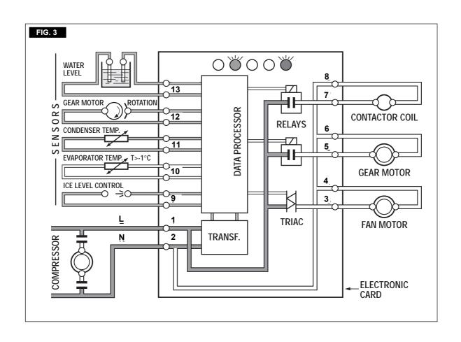
**NOTE**. If, after ten minutes from the compressor start-up, the evaporating temperature has not dropped down to a value lower than -1°C (30°F) the evaporating temperature sensor detects such an abnormal situation and stops consequently the unit
