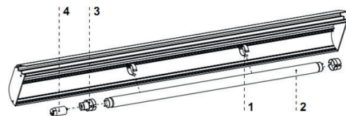
Fig.10 Changing the fluorescent lamp
